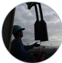
Shore Power Plugs on a Container Ship
