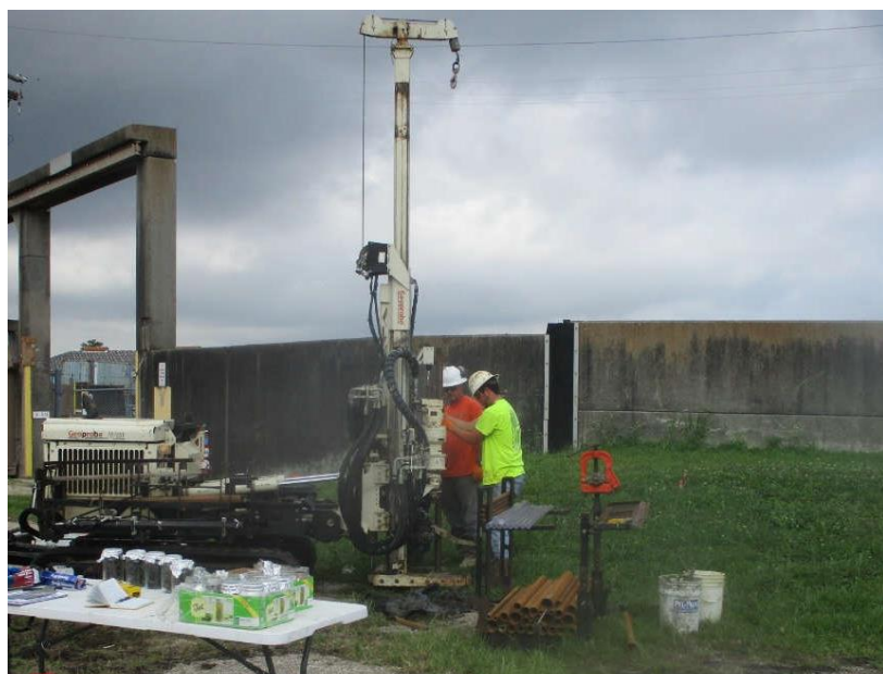
Figure 7. Consultants conducting a Phase II ESA at a PIER Plan catalyst site.
