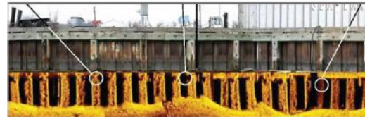
Fig. C-25. Sector scanning sonar image of steel bulkhead with typical defects circled Source: Courtesy of Collins Engineers, Inc., reproduced with permission.
