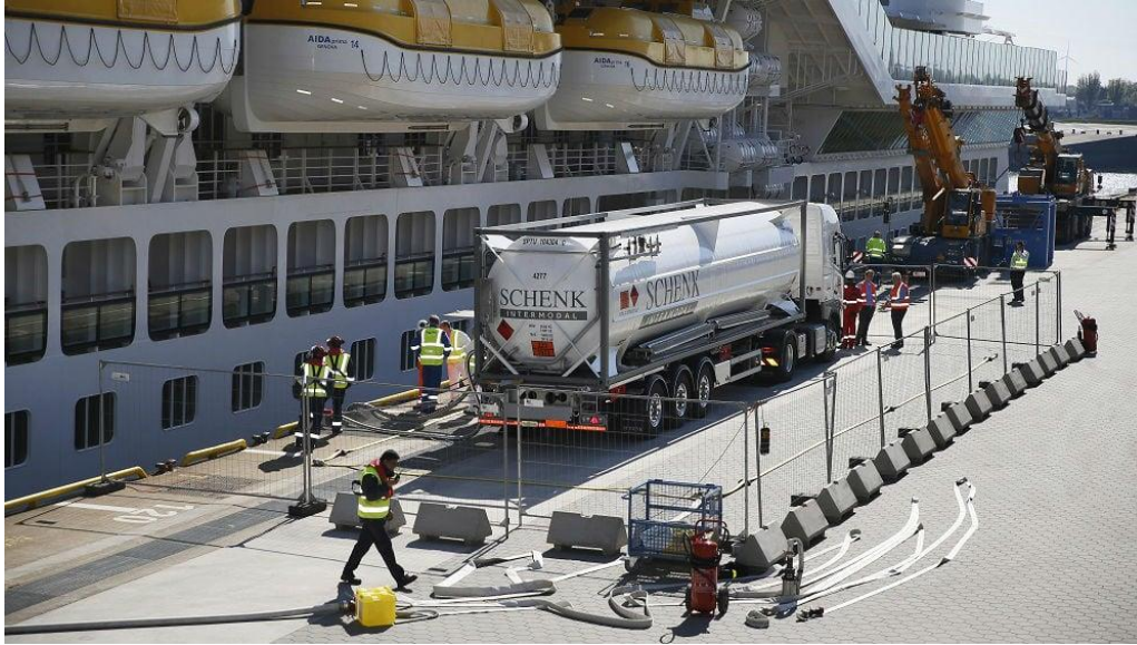
Figure 7. Liquid Natural Gas is being delivered to a cruise ship alongside the berth.
