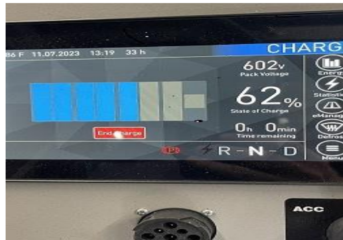
Figure 10. The battery gauge inside of the electric yard tractor shows a battery percentage of 62% after 5 hours of operation.
