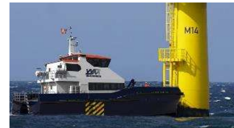
Wind CTV in position at work against an offshore wind turbine.
